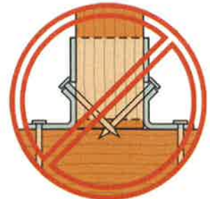
Shorter nails may not be used as double shear nails
